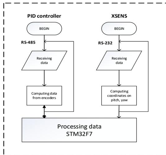
Fig.9. Processing data by PID and IMU
