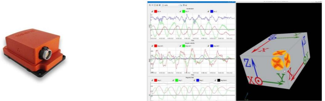
Fig.8. Inertial Measurement Unit (IMU)
