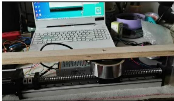
Fig. 14. The slide table is equipped with an electromagnet to control the movement of the permanent magnet
