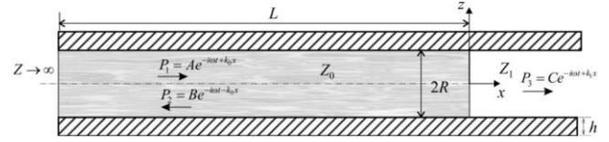
Fig. 1. A cylindrical waveguide filled with water
