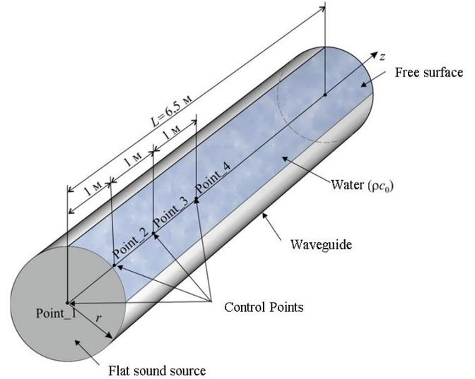
Fig. 3. Numerical model of a cylindrical waveguide
