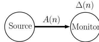
Fig. 1: A source sends status updates through a channel to a monitor. At time  $n+1$  an update is successfully received and the AoI process  $\Delta(n)$  is reset to one if the event  $A(n)$  has occurred.
