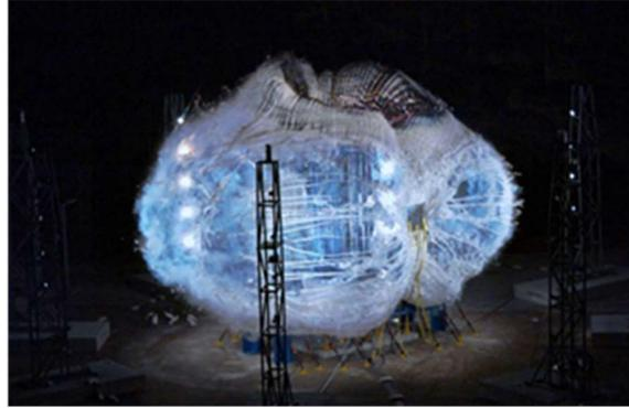
**Figure 8. Full-Scale Burst Unit #1 Captured at the Moment of Bursting.**
