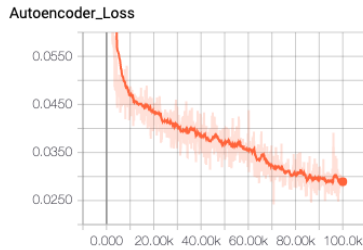
Fig. 7. Autoencoder loss - extroversion: Shows how accurately the decoder reconstructs the original input
