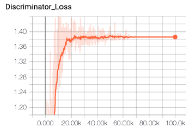
Fig. 8. Discriminator loss - extroversion: Shows how well the discriminator can separate real from fake examples
