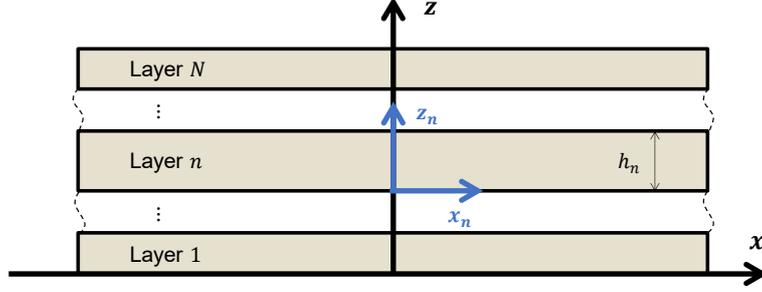
Fig. 2. Laminated composite plate
