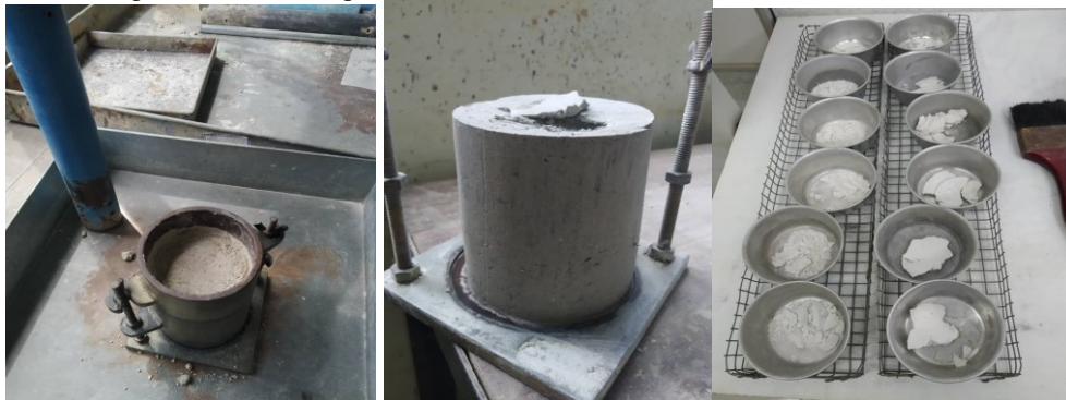
Figure 2: Process of standard Compaction Test (Compacting, Oven Dry)
