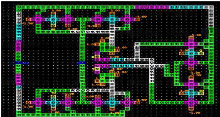
Figure 13. QCA Implementation of D Flip Flop used in Proposed Circuit.
