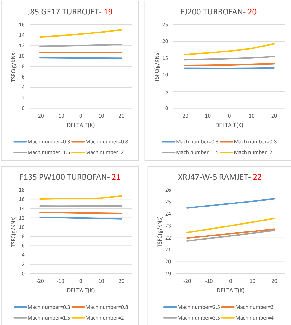
Fig. 14. TSFC changes for J85GE17 turbojet, F135 PW100 turbofan, EJ200 turbofan, XRJ47-W-5 ramjet engines at an altitude of 20,000 meters and for hydrogen fuel with changes in inlet air temperature.
