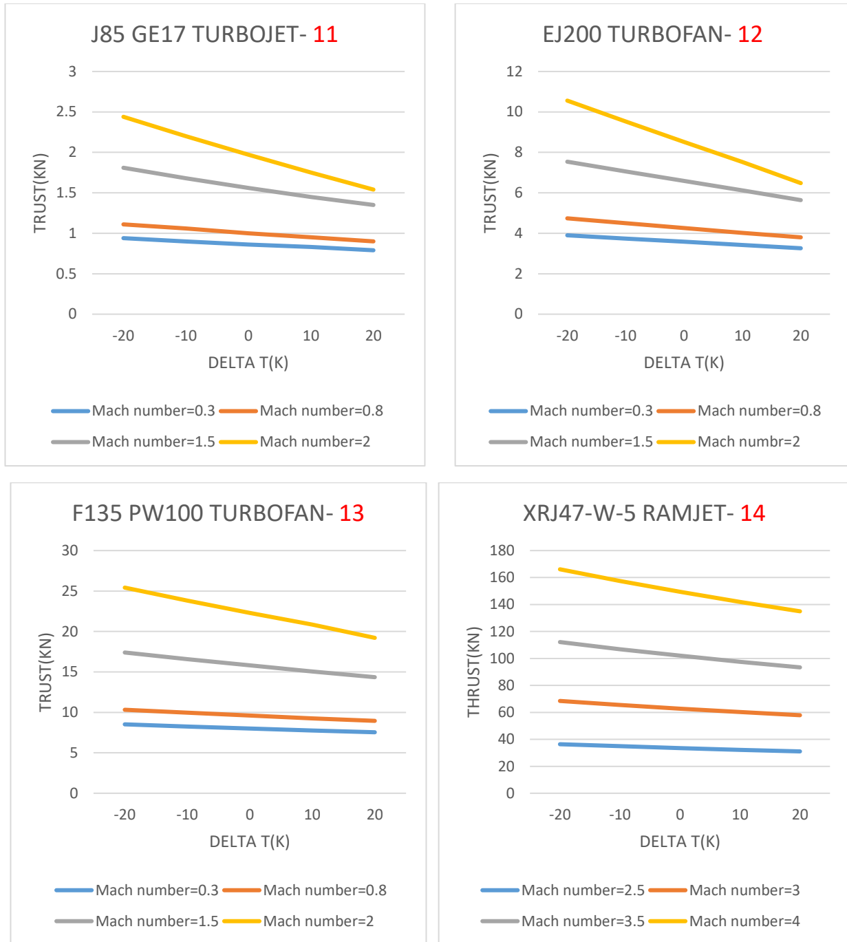
Fig. 12. Thrust changes for J85GE17 turbojet, F135 PW100 turbofan, EJ200 turbofan, XRJ47-W-5 ramjet engines at an altitude of 20,000 meters and for hydrogen fuel with changes in inlet air temperature.
