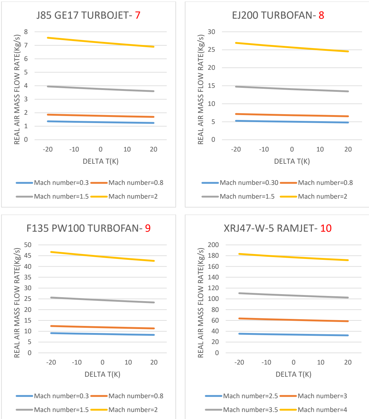
Fig. 11. changes in the actual flow rate of the inlet air for J85GE17 turbojet, F135 PW100 turbofan, EJ200 turbofan, XRJ47-W-5 ramjet engines at an altitude of 20,000 meters and for hydrogen fuel
