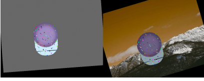
Figure 1. Depiction of image synthetic spatial augmentation and correspondences mapping in an image-pair. The colored encoded dots in the figure represents correspondences in an image-pair.
