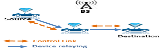
Fig. 2. D2D communication with self-controlled links.
