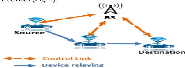
Fig. 1. D2D communication with BS controlled link.
