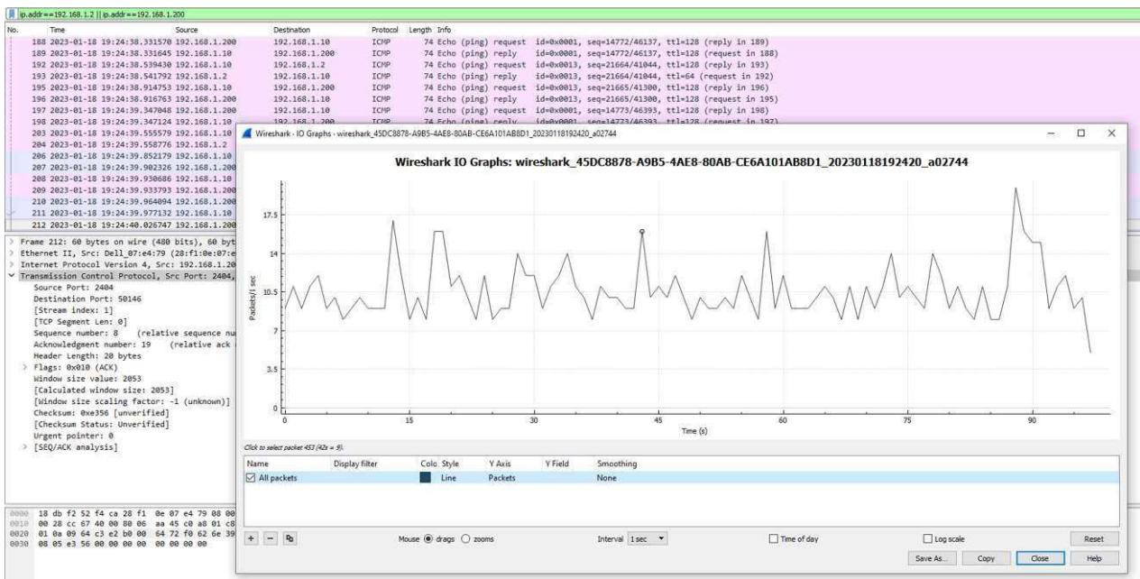
Fig 7. IO Graphs for Functional SDN based Architecture for wind farm process automation, where it show how the packet flows captured from the windsurfing server, which are around 17.5 packet/sec, all the packets are forwarded / received without any
