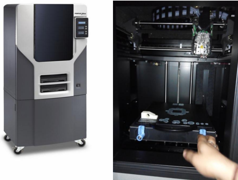
Fig. 1. FDM 250mc (Stratasys Inc.) with a specimen
