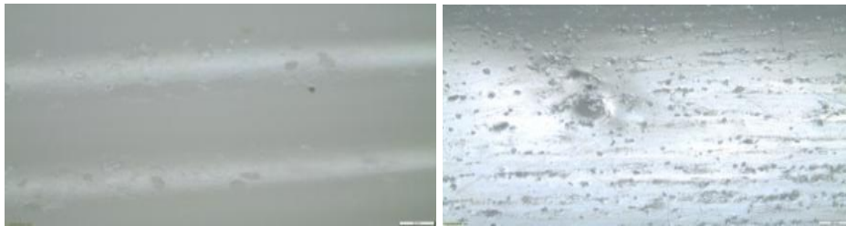
Fig. 4.2. Curved surface before (left) and after (right) Smoothing
