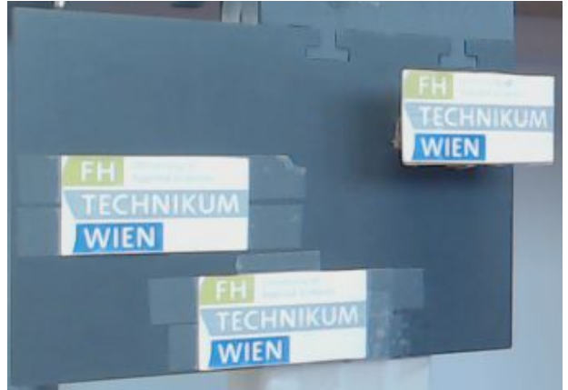
Figure 1. The visual target used for docking. The target location is on the ground in front. The origin for the PnP solvers is in the upper left corner. The logos are roughly 9x3 centimeters in size. The upper right logo was raised during experiments to remove coplanarity.
