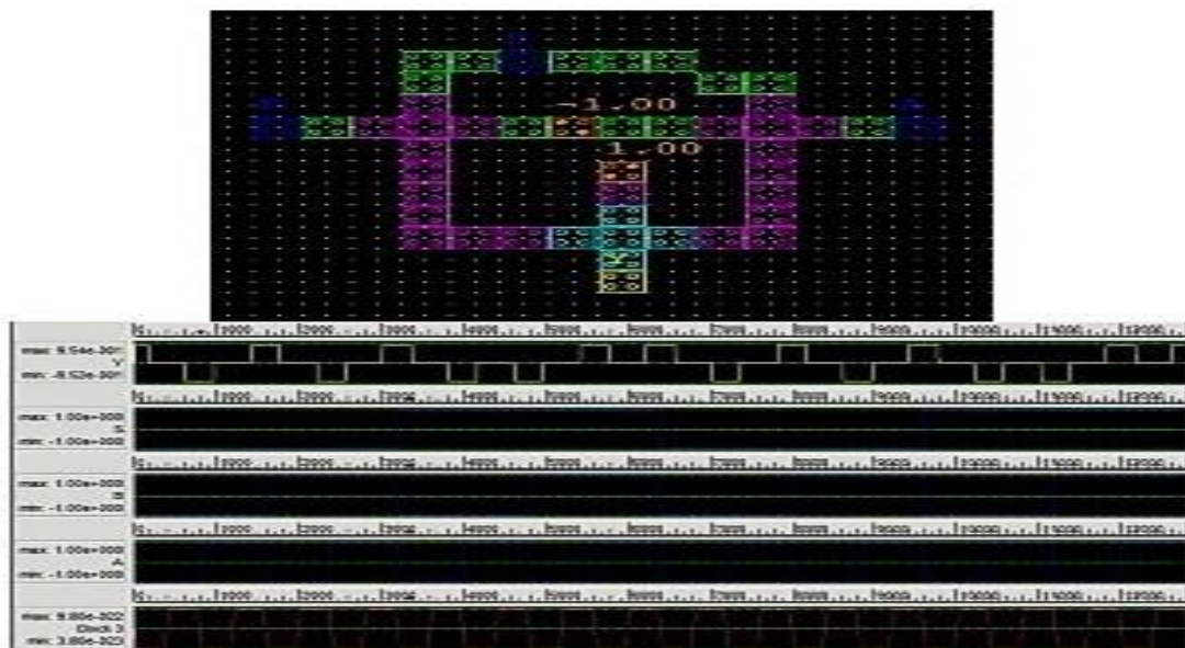
Fig. 29 Multiplexer design and simulation result
