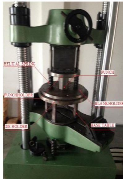
Figure 1. Deep drawing tool setup
