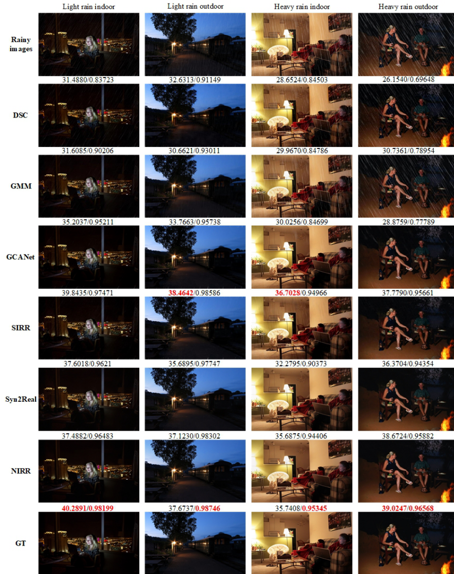
Fig. 4: Qualitative comparison and PSNR/SSIM of different methods, from the first row to the last row, the displayed pictures are the synthetic rainy images, the derained results of DSC, GMM, GCANet, SIRR, Syn2Real, our NIRR and the ground truth, respectively.
