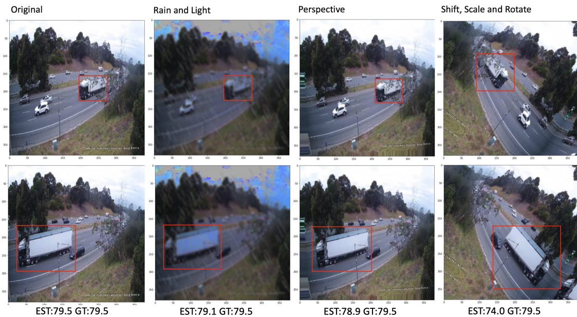
Fig. 5. Results using the Augmented Data Set. The top images are the first frame, the bottom images are the second frame; EST indicates the estimated speed and GT indicates the ground-truth speed.
