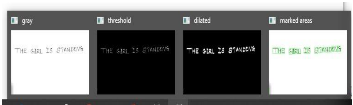
Fig 4: Input image with various pre-processing steps (gray scale, threshold, dilation)
