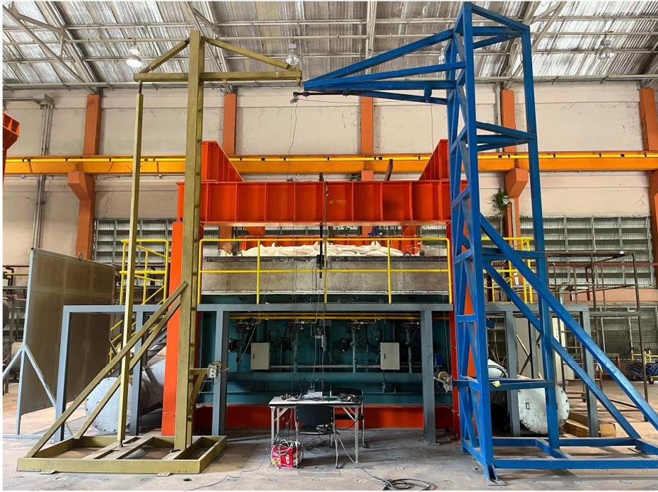
**Fig. 5** Specimen set #1 during the fire test
