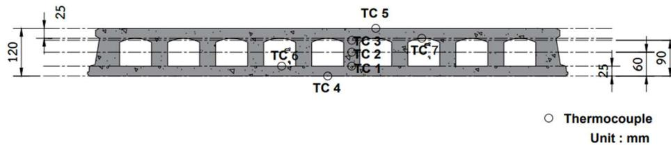
**Fig. 4** Temperature measuring devices on the cross-section of a hollow-core slab
