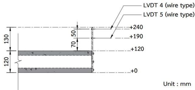
**Fig. 3** The measurement of thermal expansion
