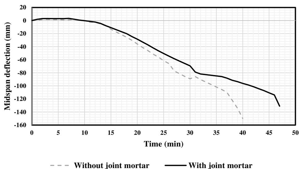
**Fig. 7** Midspan deflections measured during the fire tests
