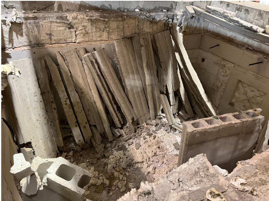
**Fig. 6** Specimen set #1 after collapse
