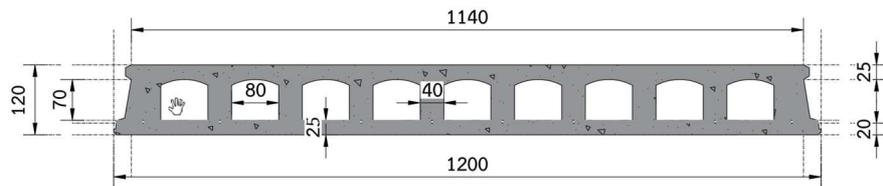
**Fig. 1** Details of the precast concrete slab (units in millimetres)
