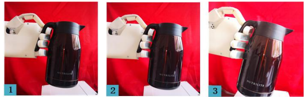
Fig.16. Demonstration of the kettle being picked up
