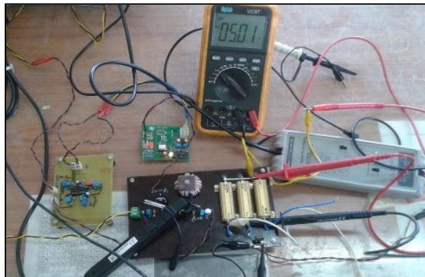
Fig. 9. Laboratory prototype of the Buck converter.
