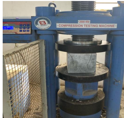
Fig. 4. Cube Specimen Compression Testing
