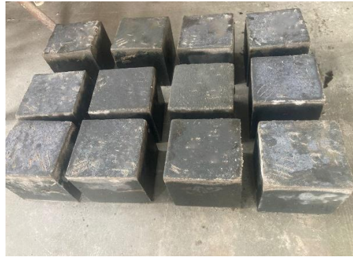
Fig. 3. Specimen Successfully Cured at Ambient Temperature.
