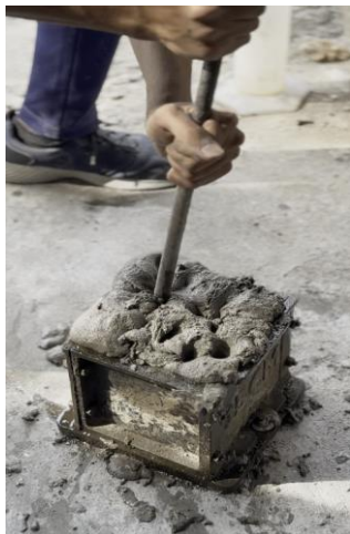
(a) Compacting concrete
