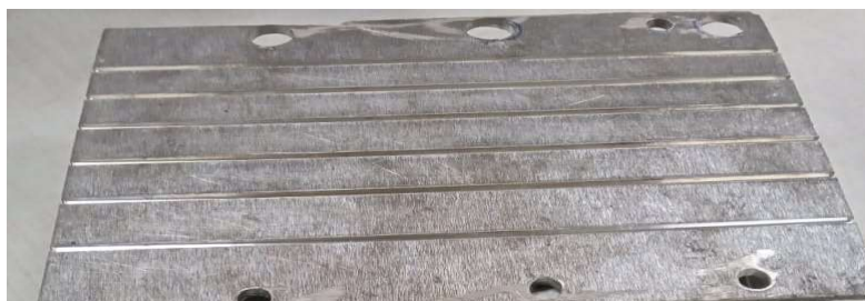
Fig.:02 Magnesium AZ31B after cutting the Grove
