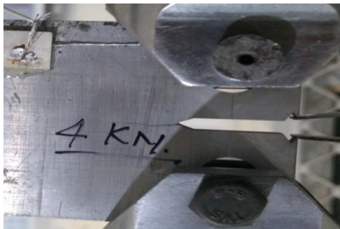
Figure 5 (a) A propagated crack in specimen during loading
