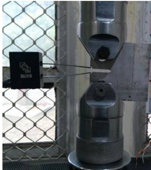
Figure 4 Specimen gripping on the test system with COD
