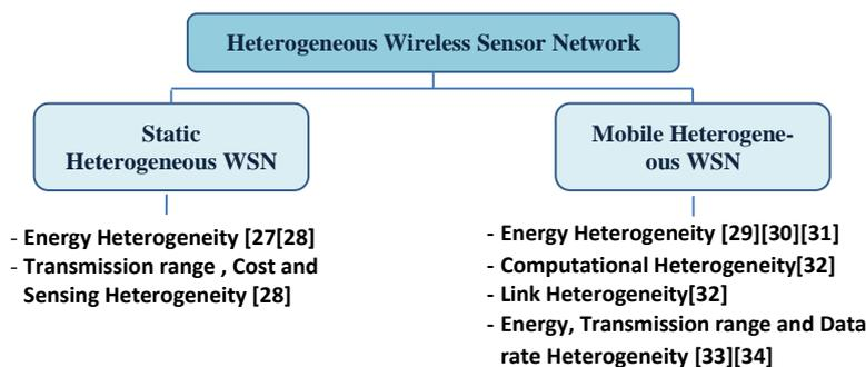
**Fig. 4:** Classification of energy-efficient Heterogeneous routing protocols based on Static and Mobile Environment
