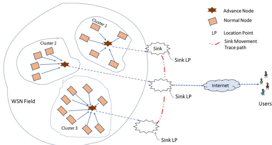
**Fig. 5:** Mobility Scenario in heterogeneous wireless sensor network
